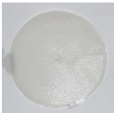
Figure 4.9. A used nanofiltration membrane (Koch MPF-50)
