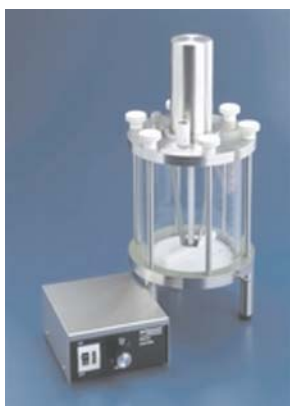
Figure 4.4. High-Output Stirred Cell from Millipore.[12]
